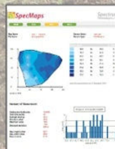
TDR 300 on a putting green: The areas with higher soil moisture are shown in deep blue.
